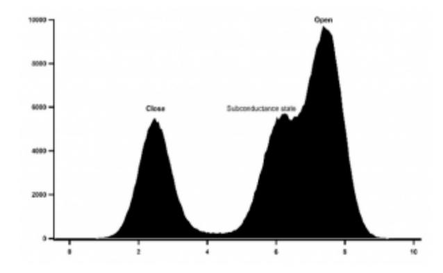
Figure 2: Histogram of mKv1.3 activity at +50mV in absence of drugs. The conductance of mKv1.3 was as well calculated using all point histogram of 1800 single channel events,  $G=98,4\pm6$  pS at +50mV. The activity showed a voltage asymmetry of the activation, with single channel activated for voltages higher than -25mV and reaching a high open probability at +50mV. Subconductance states are also observed.
